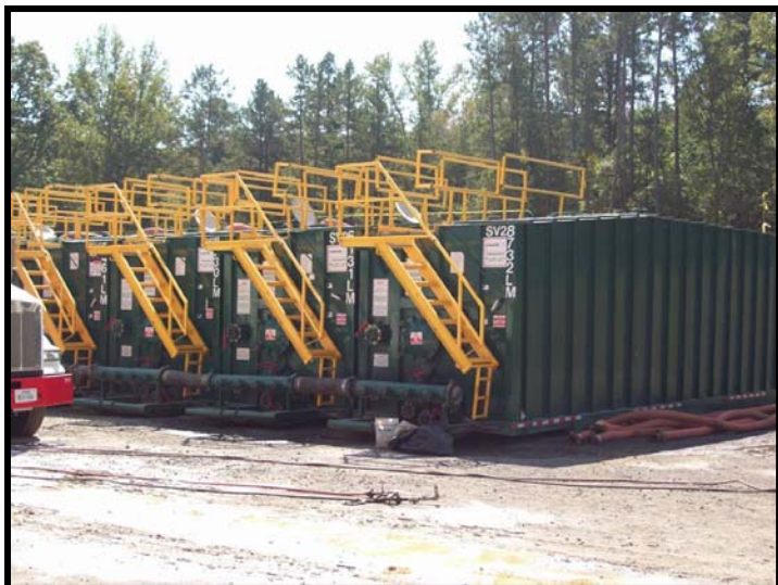
Water Storage – “Frac” Tanks (Fayetteville Shale) Source: ALL Consulting 2008
